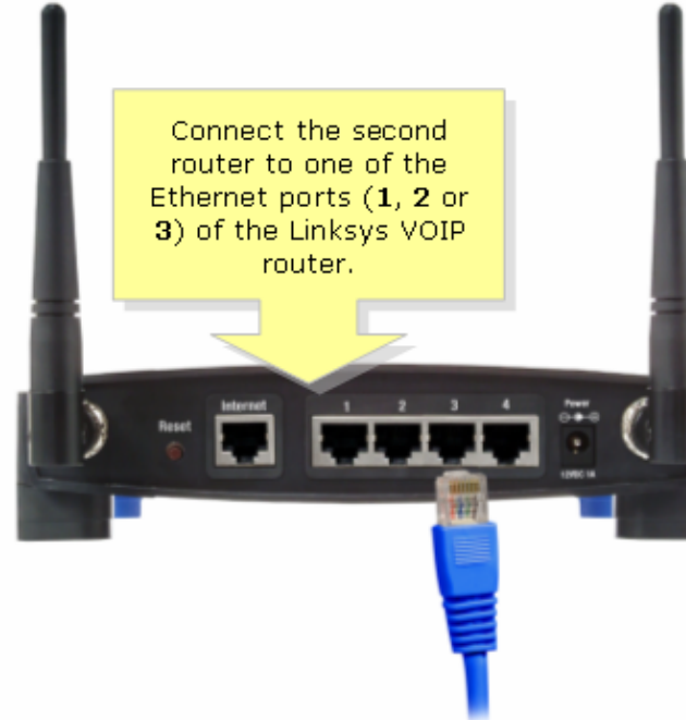
Second Router (Linksys router which will be connected to the Linksys VOIP router)
