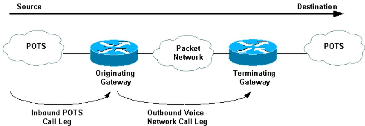
For inbound calls from a plain old telephone service (POTS) interface that are destined for the packet network, the originating router/gateway matches an *inbound* POTS dial peer for the *inbound call leg* first. Next, the originating router/gateway creates an outbound Voice–Network dial peer such as Voice over IP (VoIP) or Voice over Frame relay (VoFR) for the *outbound call leg*. After this, the router/gateway bridges the two call legs.
