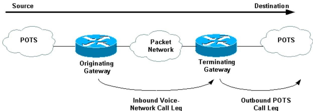
For inbound calls from a Voice Network interface that are destined for a POTS interface, the terminating router/gateway matches an *inbound* Voice Network dial peer for the *inbound call leg*. Next, an outbound POTS dial peer is created for the *outbound call leg*.
