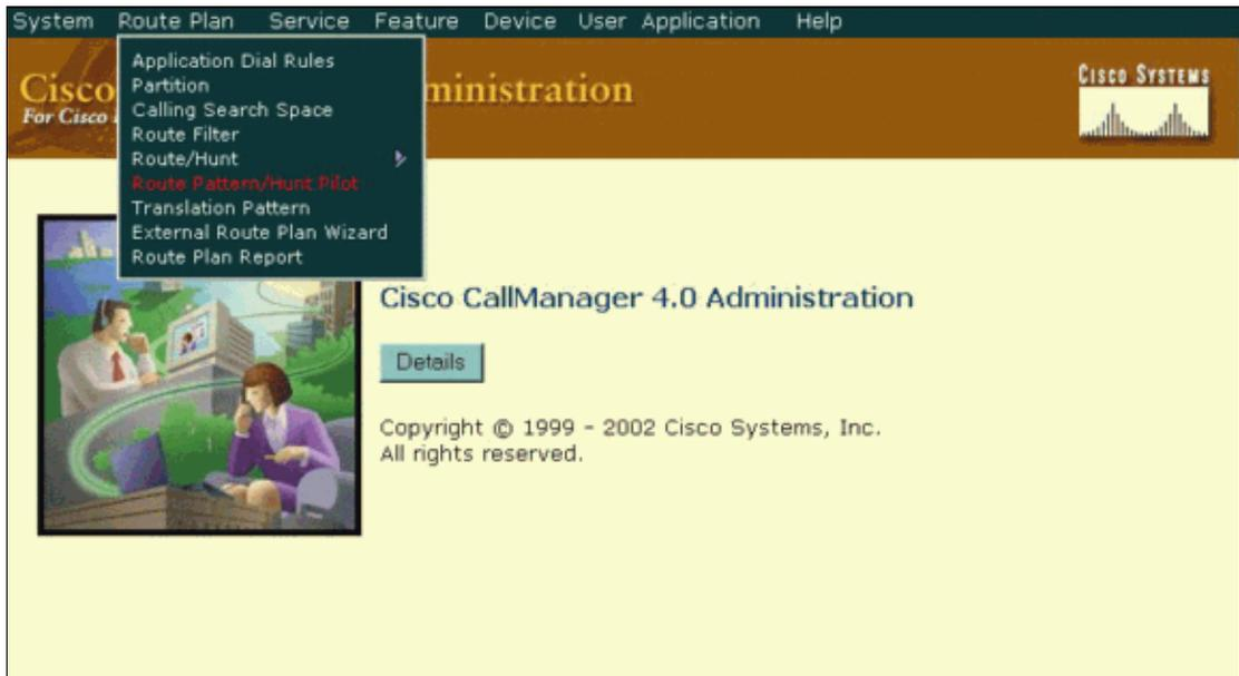
2. Specify the values used to route calls to the H.323 gateway in the Route Pattern/Hunt Pilot Configuration window.
