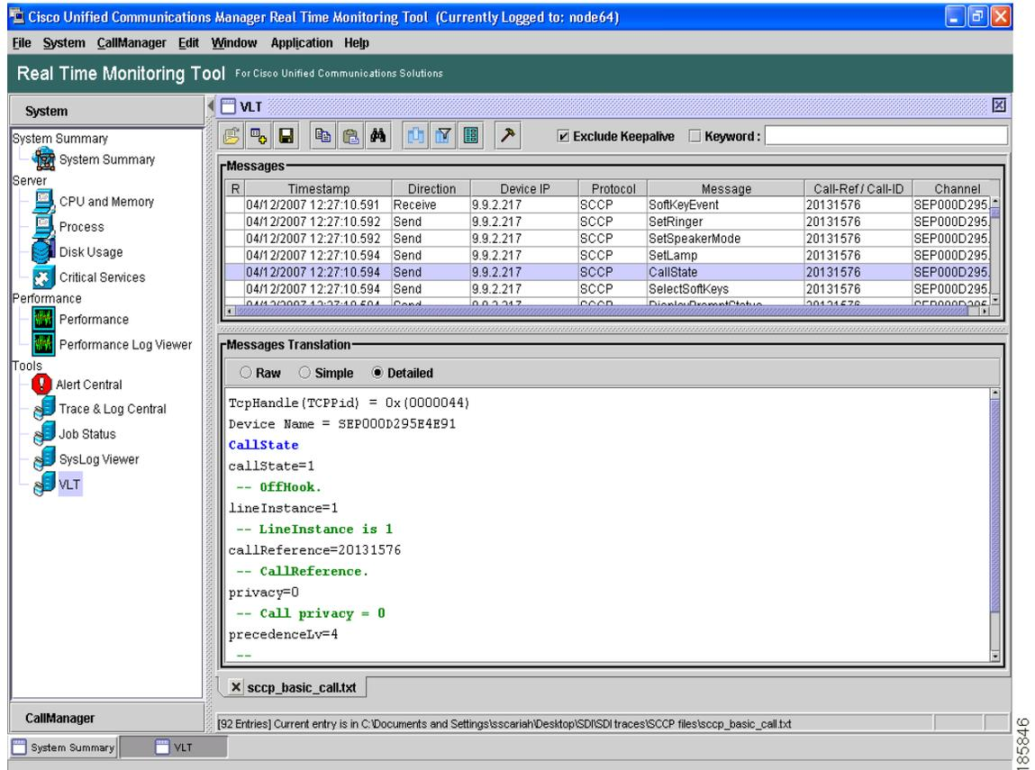
The window allows for typical GUI display control such as window resize, column resize, vertical and horizontal scroll, minimize, restore, and close. You can also grab and move the border between the Messages upper pane and the Messages Translation lower pane.
