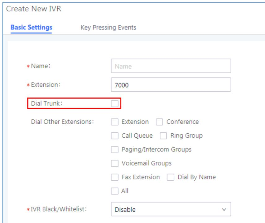
The screenshot shows the 'Create New IVR' configuration page. The 'Basic Settings' tab is active. The 'Dial Trunk' checkbox is highlighted with a red border and is currently unchecked. Other visible settings include:
