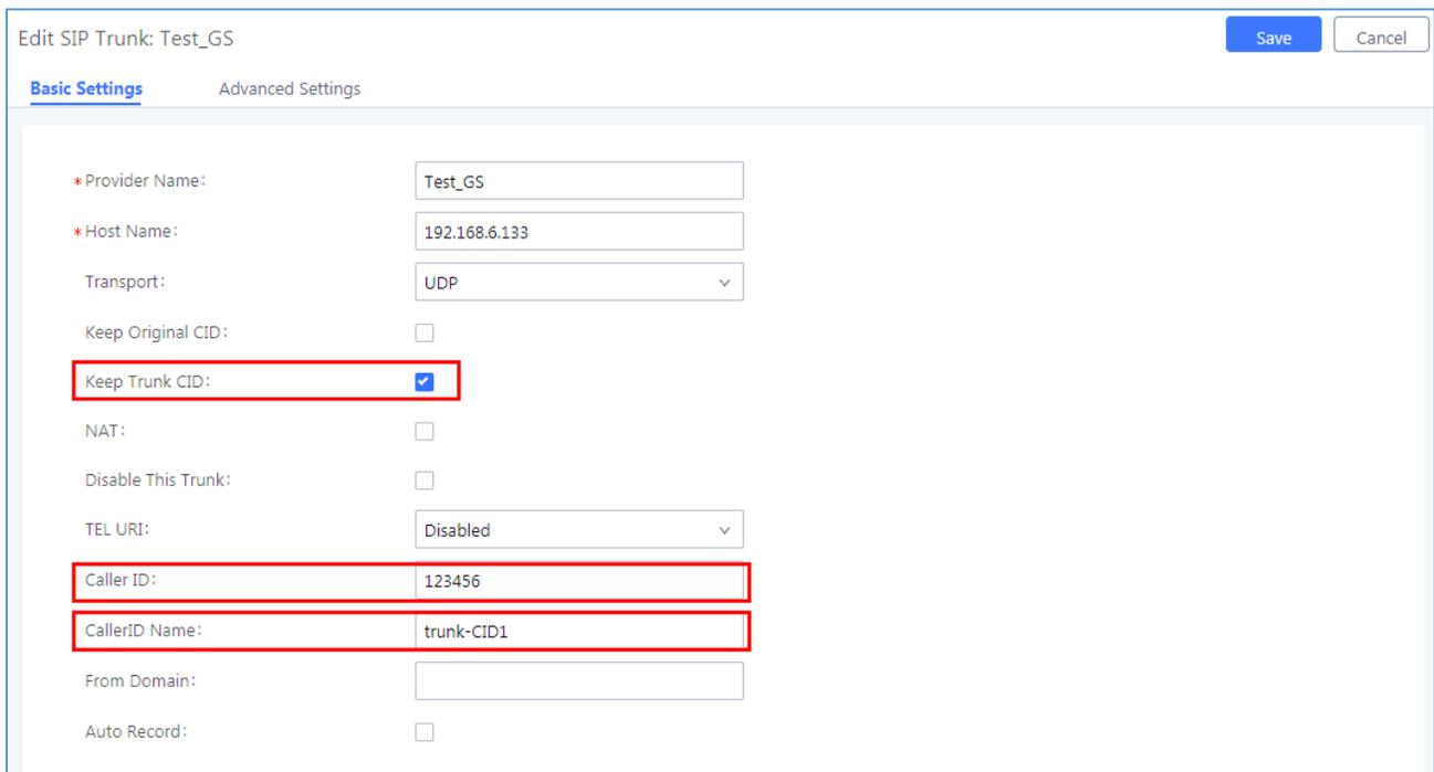
Figure 8 shows the configuration for a SIP Trunk. The 'Basic Settings' tab is selected. The 'Keep Trunk CID' checkbox is checked, and the 'Caller ID' and 'CallerID Name' fields are highlighted with red boxes. The configuration values are as follows:
