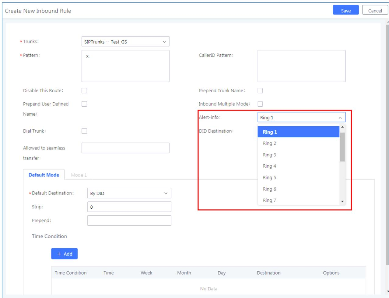
The screenshot shows the 'Create New Inbound Rule' configuration page. The 'Alert-info' dropdown menu is open, showing a list of ringtone options from 'Ring 1' to 'Ring 7'. 'Ring 1' is currently selected and highlighted in blue. Other fields visible include 'Trunks' set to 'SIPTrunks -- Test\_GS', 'Pattern' as '\_x.', and 'Default Destination' as 'By DID'.
