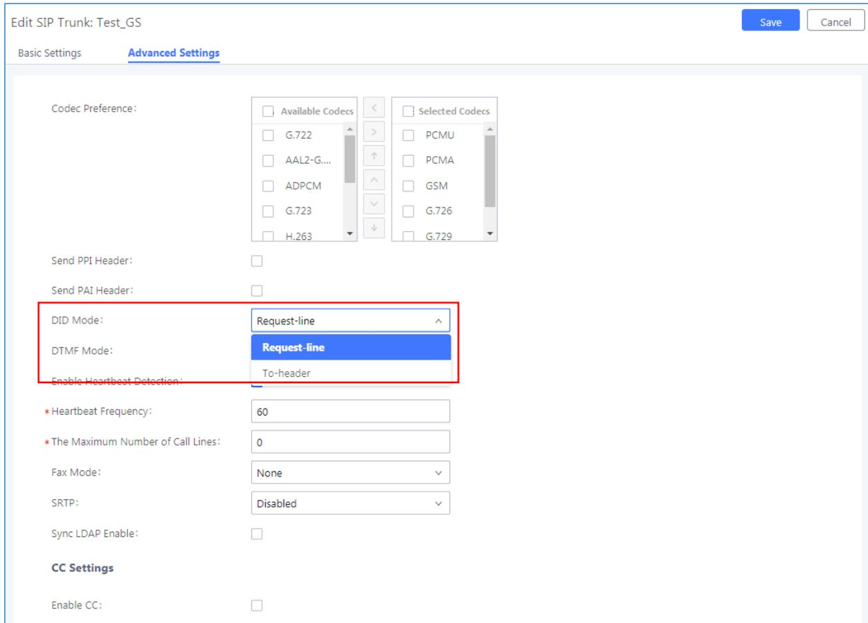
The screenshot shows the 'Edit SIP Trunk: Test\_GS' configuration window. The 'Advanced Settings' tab is active. The 'DID Mode' dropdown menu is highlighted with a red box and shows 'Request-line' selected. Other settings include:
