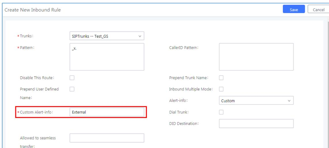
The screenshot shows the 'Create New Inbound Rule' configuration page. The '\* Custom Alert-info' dropdown menu is highlighted with a red box and set to 'External'. Other fields visible include 'Trunks' set to 'SIPTrunks -- Test\_GS', 'Pattern' as '\_x.', and 'Alert-info' set to 'Custom'.
